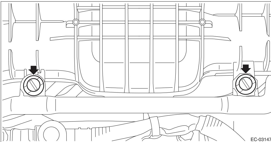
6) Remove the A/C compressor. <Ref. to AC-45, REMOVAL, Compressor.>
